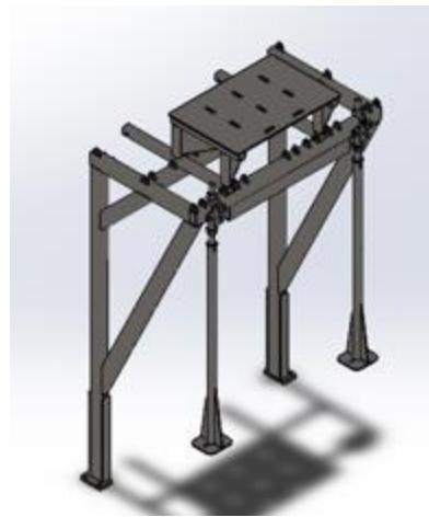
6. Attach the braces from the front support bar lug and fasten them to the ripped tube of the car.
