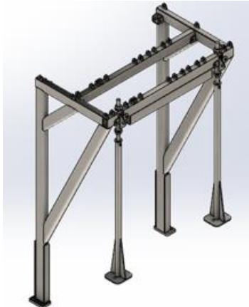
5- Fit the platform in such a way that it faces the machine bedframe.
