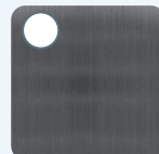
X16: AISI 316 SB Scotch Brite
